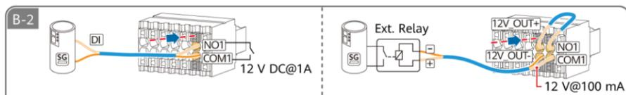
The signal DO is connected to the SG Ready heat pump.
