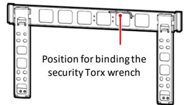
Position for binding the security Torx wrench
