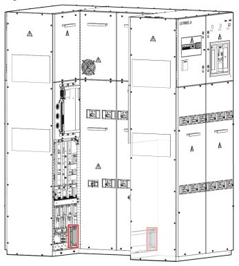
Figure 6-42 Position of the JUPITER-9000K-H1 heater
