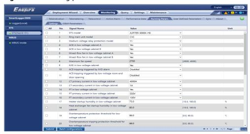
Figure 6-56 Viewing teleindication signal parameters
