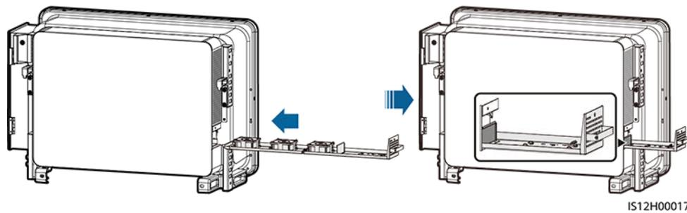
**Step 9** Connect the cables correctly according to the cable labels and bind the cables.
