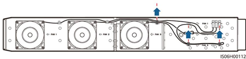
**Step 5** Remove the faulty fan (FAN 1 is used as an example).
