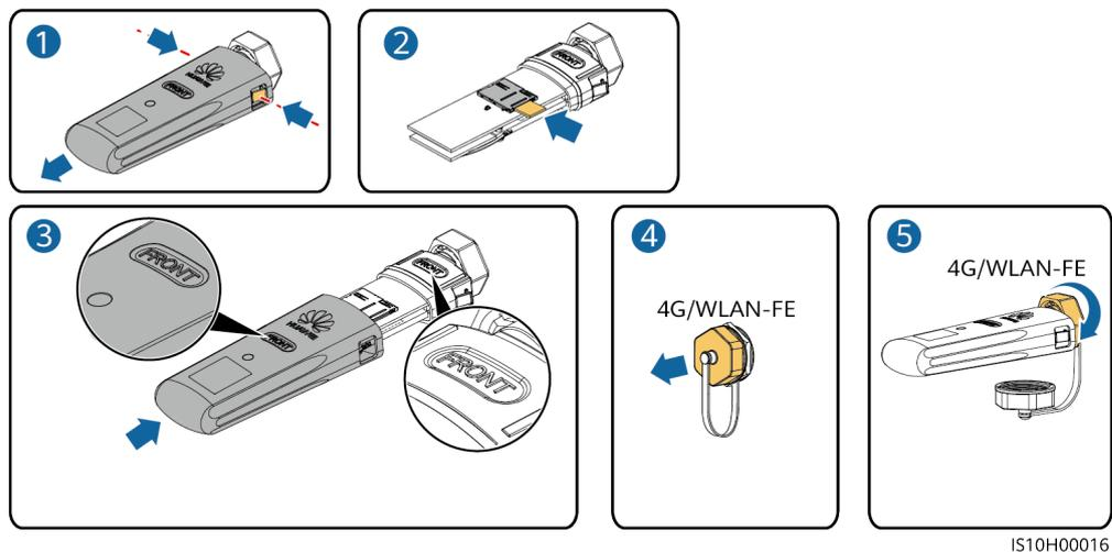
**Figure 5-35** Installing a 4G Smart Dongle (SDongleB-06)
