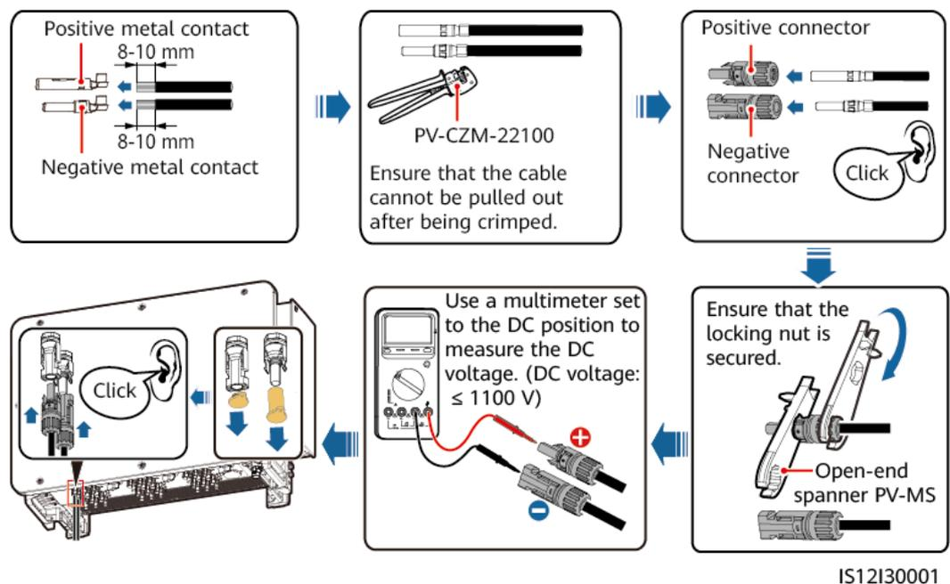
Figure 5-29 Connector connection
