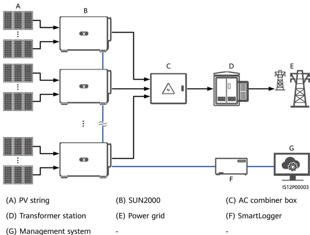
**Figure 5-2 RS485 networking (SDongle)**
