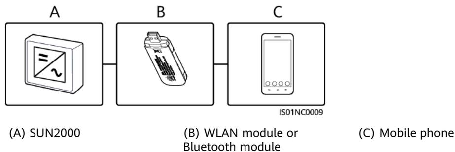
**Figure 7-2** Connection over a Smart Dongle
