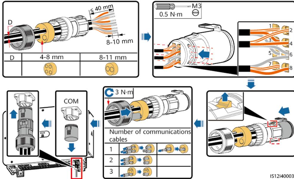
**Figure 5-33** Connecting RS485 communications cables (4–8 mm two-hole or three-hole rubber plug)
